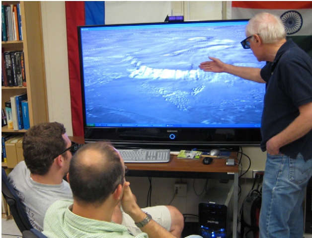
Fig. 1. A stereo capable Samsung 61" display as part of a Personal Powerwall being used to explore DTM data with the ADVISER Desktop application.
