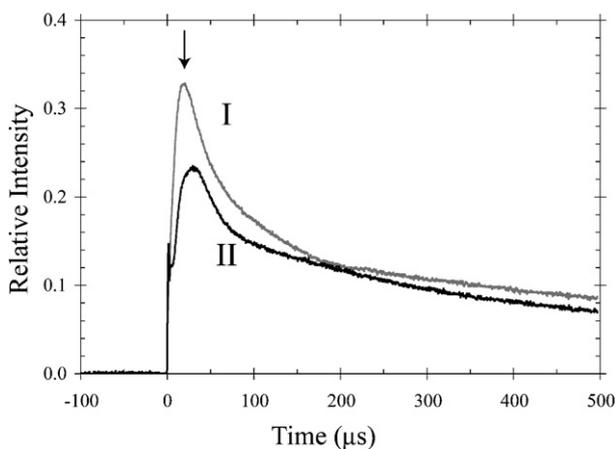
Fig. 10. The first 500  $\mu\text{s}$  light intensity curves of impacts I (gray) and II (black) from Fig. 9. The signals look different at early times, and begin to converge at later times. There is an early-time spike in the impact II signal, followed by a brief intensity decrease before the eventual intensity peak. The arrow represents the time at which Fig. 9b images were taken.
