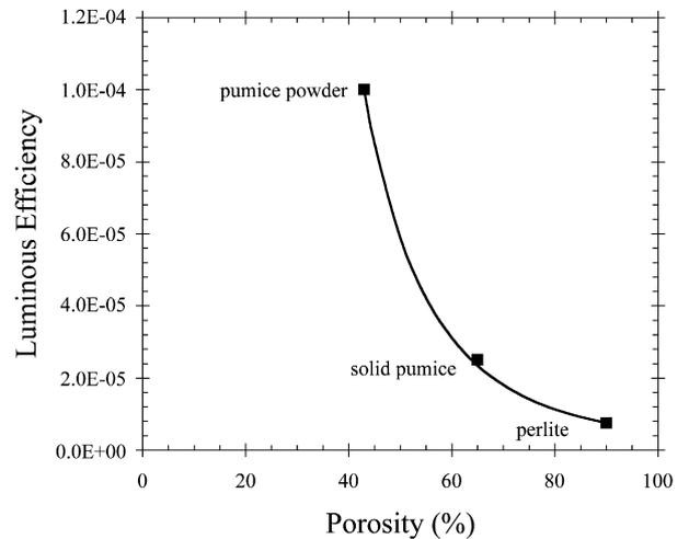
Fig. 7. Plot of the relationship between target porosity and luminous efficiency based on laboratory impacts into silicate targets (pumice powder, solid pumice, and perlite granules). The trendline represents the exponential relationship detailed in Eq. (4).
