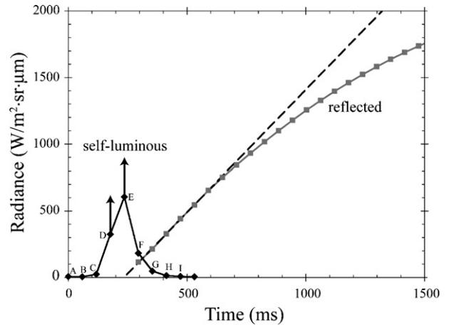
Fig. 4. Plot of the light intensity evolution of the first 1500 ms of the Deep Impact collision. The black curve represents the self-luminous (impact flash) portion of the light output. The intensity values for the saturated images represent minimum values. The gray curve represents the light reflected off of the expanding ejecta cloud. The dashed line is the initial linear growth trend of the reflecting portion extrapolated through time. The letters correspond to those from Fig. 2.
