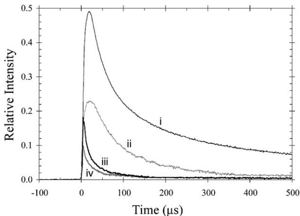
Fig. 6. Plot of the light intensity evolution of experimental impacts into targets of different porosity and volatile content. Both increasing porosity [seen in the difference between the pumice powder (a), solid pumice (b), and perlite granule (c) targets] and increasing volatile content [seen in the difference between the pumice powder (a) and dolomite powder (d) targets] lead to a suppression of the luminous output of an impact.
