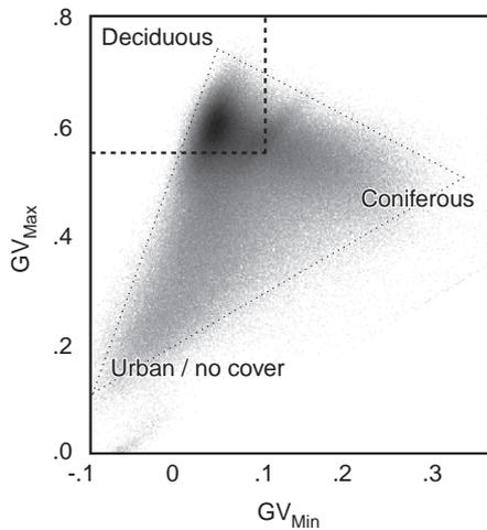
Fig. 4. Scatter plot of  $GV_{min}$  vs.  $GV_{max}$  demonstrating natural ternary spread of data. Boundaries chosen in this study to conservatively identify deciduous forest are shown. Pixels obtaining average  $GV_{max} \geq 0.55$  and  $GV_{min} \leq 0.1$  were defined as deciduous forests.
