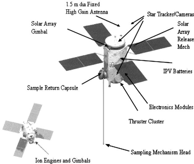
Fig. 1. The Hera spacecraft in a concept drawing by SpaceWorks (Jeff Preble) and according to mission design by Glenn research Center (Leon Gefert).
