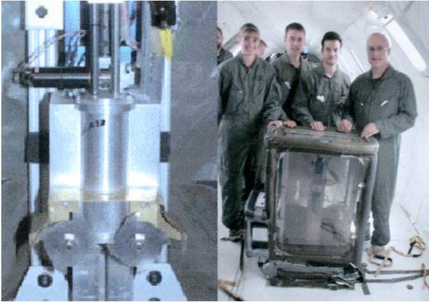
Fig. 4. (Left) The head of the Honeybee sample collector. The collector consists of two counter-rotation cutters that throw samples into a containment vessel with a closing door. (Right) The collector test fixture on board the NASA KC-135 microgravity test facility. With experimenters Melissa Franzen (University of Arkansas), Paul Bartlett (Honeybee Robotics), John DiPalma and Jeff Preble (both SpaceWorks).
