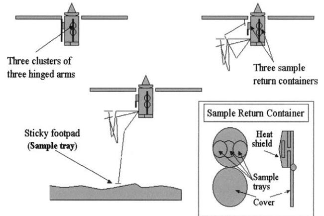
Fig. 5. The SpaceWorks sticky footpad collector. Three sets of 3 arms are associated with sample return containers. Each has a 30 cm diameter tray containing adhesive which is momentarily touched onto the asteroid surface. After collection, the sample tray is placed inside the sample return container.
