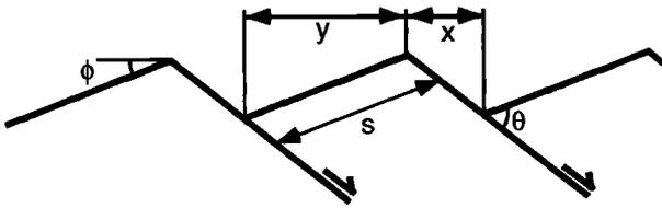
**Figure 3.** Geometric model of tilt-block extension along planar faults to derive an estimation of strain. The slope widths  $x$  and  $y$  are measured as viewed from directly above the surface,  $s$  is the fault spacing on the undeformed surface,  $\theta$  is the initial fault dip, and  $\phi$  is the tilt of the original surface. See equations (1) and (2).
