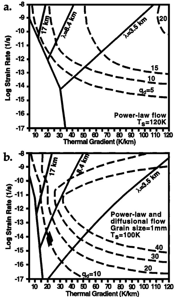
**Figure 4.** (a) Graph of strain rate vs. thermal gradient (after Herrick and Stevenson [1990]) showing contours of dominant wavelength  $\lambda$  and amplification factor at that wavelength  $q_d$  of the extensional instability. (b) Similar graph showing the effect of new flow law for ductile ice (after Dombard and McKinnon [1996]). The shaded area represents the ranges of  $\lambda$  and  $q_d$  estimated for the Uruk Sulcus stereo area.
