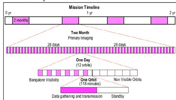
Figure 2. M3 data acquisition periods during a nominal Chandrayaan-1 mission timeline.
