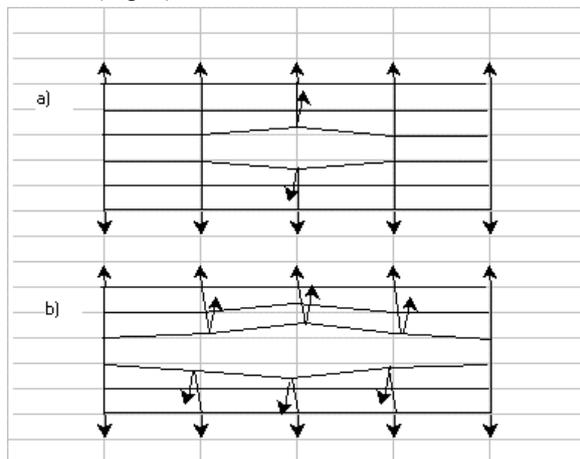
Fig. 3. Influence of Coriolis force on crack trajectory.
