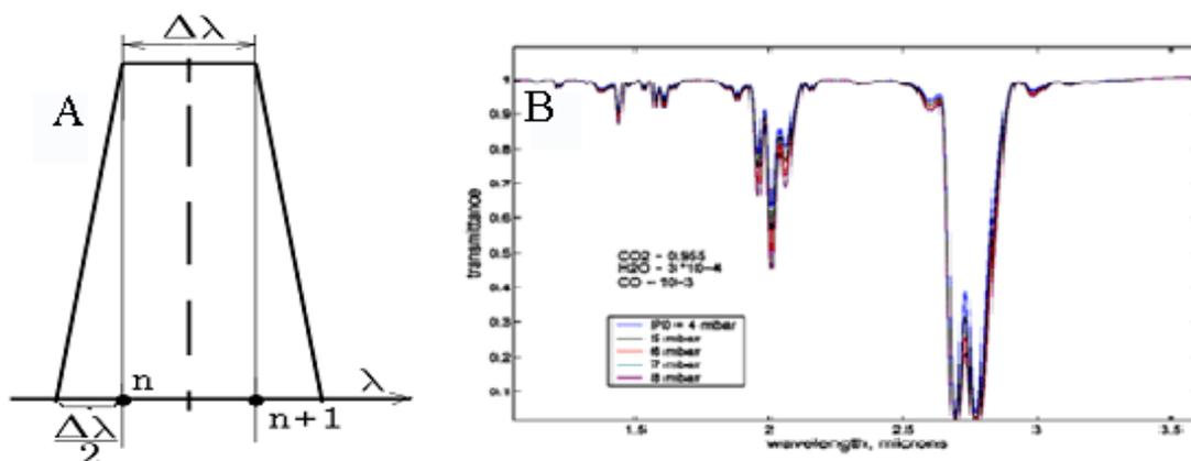
**Figure 1. Instrumental function (a) and simulated transmittance (b) used to correct OMEGA spectra on atmospheric absorption.  $n$  is pixel number,  $\Delta\lambda$  - distance between pixels in spectral scale.**
