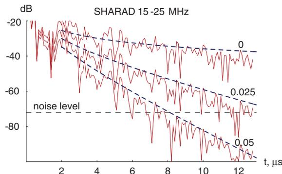
Simulated signals [12] for the northern polar cap are shown in the figure. Solid and dashed lines represent the exact solutions of electromagnetic equations and the asymptotic solutions of the radiative transfer theory. Mean loss tangents of the dust are labeled nearby the curves.
