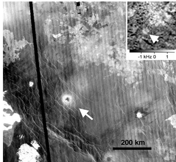
**Fig. 2.** Magellan SAR mosaic of Rusalka Planitia (2°S, 164°E). Inset shows the Doppler centroid map of the same area. Arrow shows a splotch with a well-pronounced anisotropy signature.
