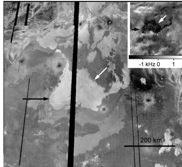
**Fig. 1.** Magellan SAR mosaic of Sedna Planitia (50°N, 345°E). Inset shows the Doppler centroid map of the same area. Arrow shows a radar-bright (rough) lava flow with a well-pronounced anisotropy signature.
